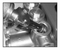
7. Use a small slide hammer to remove valve seats (37) from manifold (29). Inspect valve plate (36) and valve seats (37) for wear. If excessive pitting is seen, replace the worn parts. Check valve seat o-ring (38) for wear and replace as necessary.
